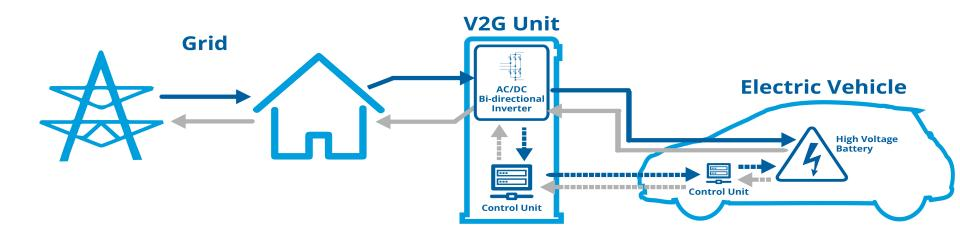
**Vehicle-to-grid (V2G)** chargers allows a two-way flow of electricity between the car and the charger and the electricity grid. This enables cars to return unused electricity back onto the charger and subsequently return it back to the grid opening up the potential for electric vehicles to become portable energy storage.
